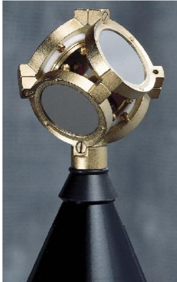
Figure 1 - The practical tetrahedral microphone (left) and design from patent document (right) which more clearly reveals its structure
