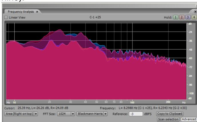
As the spectrogram left indicates, the **Mach ONE** process extends digital resolution by two bits (12dB) in the three-octave range between 20Hz to 160Hz. (The forward trace is with **Mach ONE** engaged.) Measuring the rumble performance according to DIN(A) or NAB, the unweighted rumble signal improves by 10dB to 18dB depending on the test disc employed.
