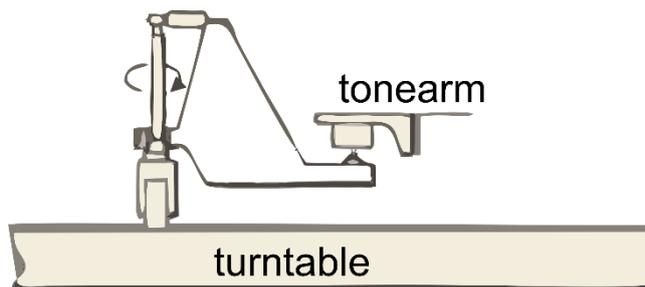
The reproducing stylus is placed on the tiny, black, PVC platform on the lower arm of the swivelling boom-frame (see diagram left).
