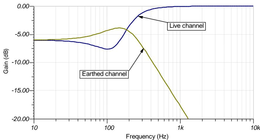
The transfer function to the two output ports is given in the graph (left). The inevitable non-constant group-delay response of this type of circuit leads to amplitude-response anomalies: in this case the 2dB “bump and dip” around 150Hz.
