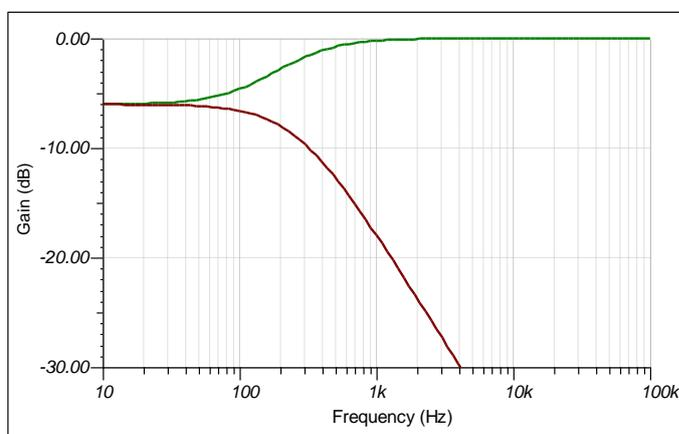
The default circuit values of the resistances and inductor in the Neumann equipment result in the transfer functions illustrated in the graph left (to both output ports, one input driven, the other grounded). They indicate the effect of the unit is not subtle.<sup>44</sup> The “live” channel is gradually attenuated below about 500Hz so that only a few dB of separation exists at 100Hz.
