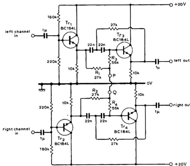
Of course, we are not the first to have considered this technique. The earliest reference we have is from *Wireless World* magazine *Circuit Ideas* from 1975; the very apogee of the vinyl record and firmly in the era of analogue electronics (shown left).<sup>39</sup>
